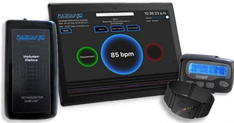
What it is: The PulseGuard™ Mk-II system consists of two components: a lightweight watch type sensor that communicates via Bluetooth with the PulseGuard™ Software installed onto your own approved tablet.
