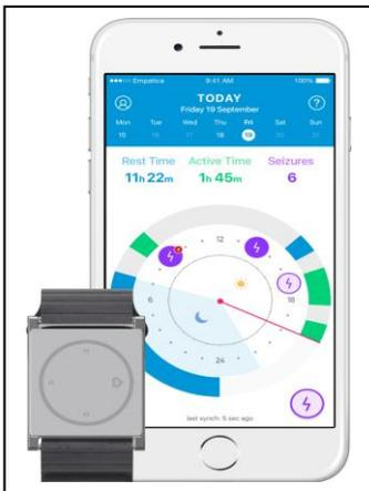
**What it is:** A smartwatch created in the USA that is connected to a person's mobile via Bluetooth connection which may detect tonic clonic seizures and can monitor activity levels and sleep quality. It can also act as a seizure diary. When it detects a tonic clonic seizure, it will send an alert SMS to caregiver's phones. It is also able to detect the location of an individual to help a care giver to respond to a potential seizure crisis.
