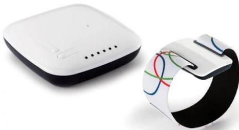
What it is: A comfortable wireless armband that closely monitors heart rate and motion while the wearer is lying in bed. When the NightWatch detects a potentially severe seizure, a warning is transmitted to a caregiver via a wireless signal to the armband's corresponding base station.
